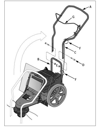
Figure 2-2: Handlebar installation.
